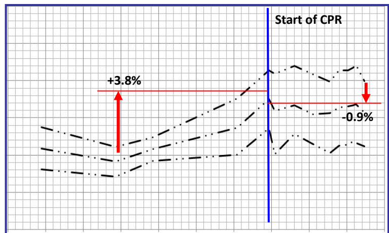
Figure 3: Aging of the plant in terms of SPC (kWh/t NaOH)
